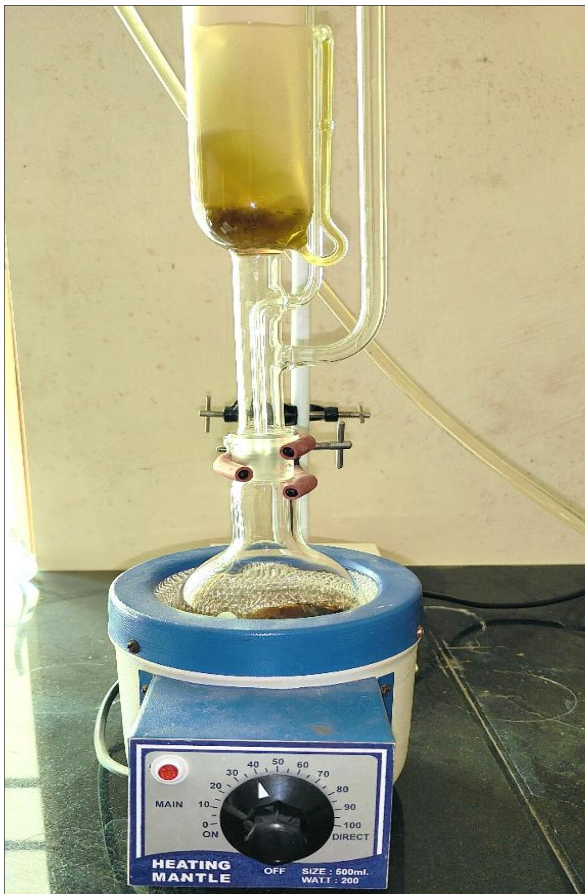
Figure 2: Soxhlet extraction of experimental plant sample
